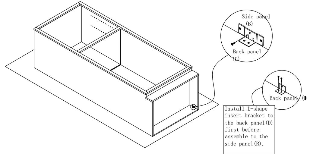
Step 9 : Install corner block. Install rainbow bracket to the side panel (B), front frame (A) and back panel (D) with the (3)Ø3.5x16mm screw.
