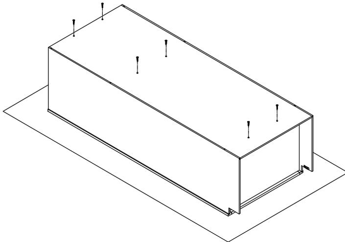
Step 6 : Fit in the L-shape insert bracket from front frame (A) into bottom panel (C) bracket and screw the bracket with(3)  $\varnothing 3.5 \times 14$ mm screw.
