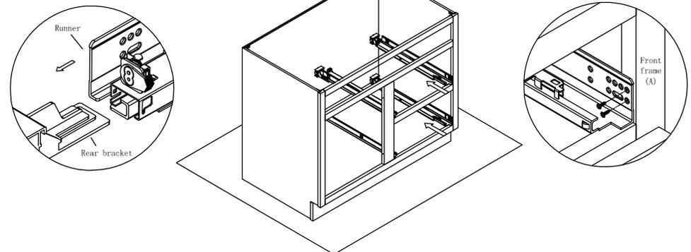
Step 11 : Put the drawer box on the drawer slide and push the drawer box to make the end of runner is lock to the hole of the drawer back panel. Complete the installation of the drawer box when you hear sound click which mean the locking device is locked on the drawer slide.
