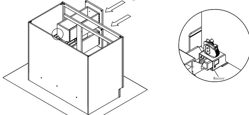
Step 12 : Install door panel (G). Screw the hinge to the front frame (A) and door (G).
