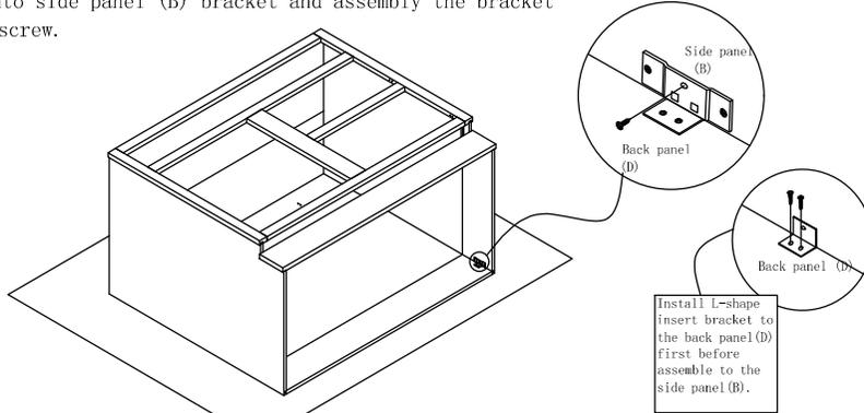
Step 8 : Install corner block. Install rainbow bracket to the side panel (B), front frame (A) and back panel (D) with the (4)  $\varnothing 3.5 \times 16$ mm screw.
