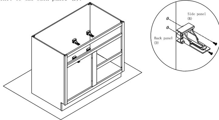
Step 10 : Insert drawer slide runner to the rear slide bracket and screw the drawer slide to the guide hole of front frame (A) and hole for drawer slide
