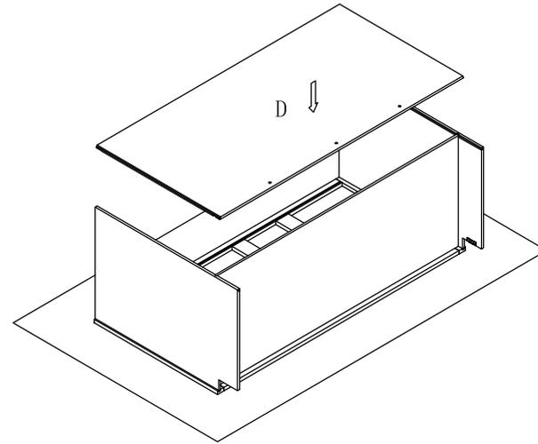
Step 5 : Install screw(5)  $\varnothing 3.5 \times 35 \text{mm}$  into back panel (D).
