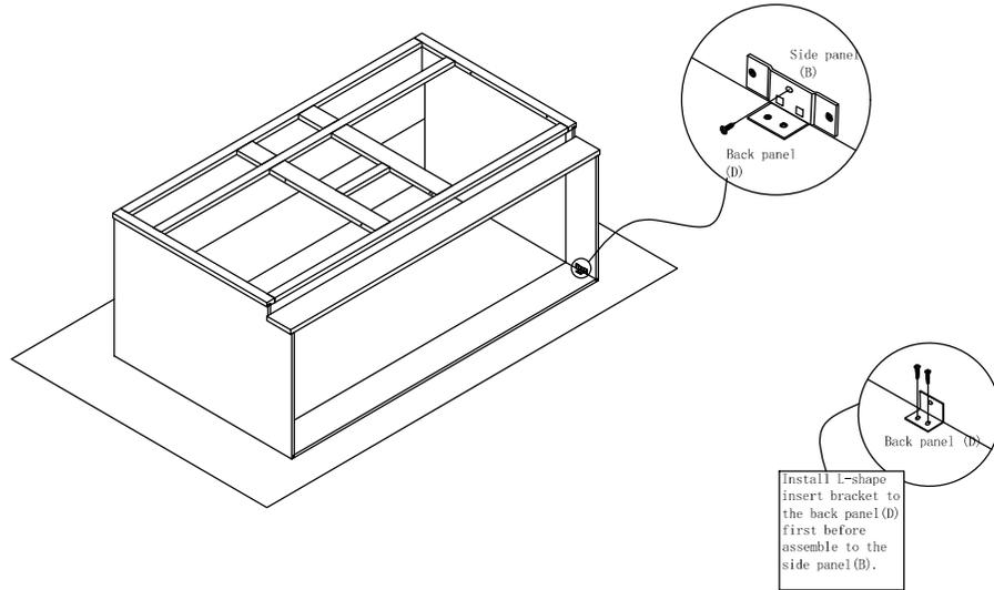
Step 8 : Install corner block. Install rainbow bracket to the side panel (B), front frame (A) and back panel (D) with the (4)  $\varnothing 3.5 \times 16$ mm screw.
