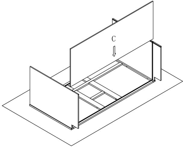
Step 4 : Install back panel. Insert back panel (D) into groove of left and right side panel(B).
