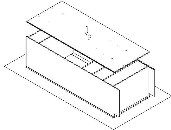
Step 5 : Install assembly screws(5)  $\varnothing 3.5 \times 35$ mm into back panel (D) then fit in the L-shape insert bracket from front frame (A) into bottom panel (C) bracket and screw the bracket with(3)  $\varnothing 3.5 \times 14$ mm screw
