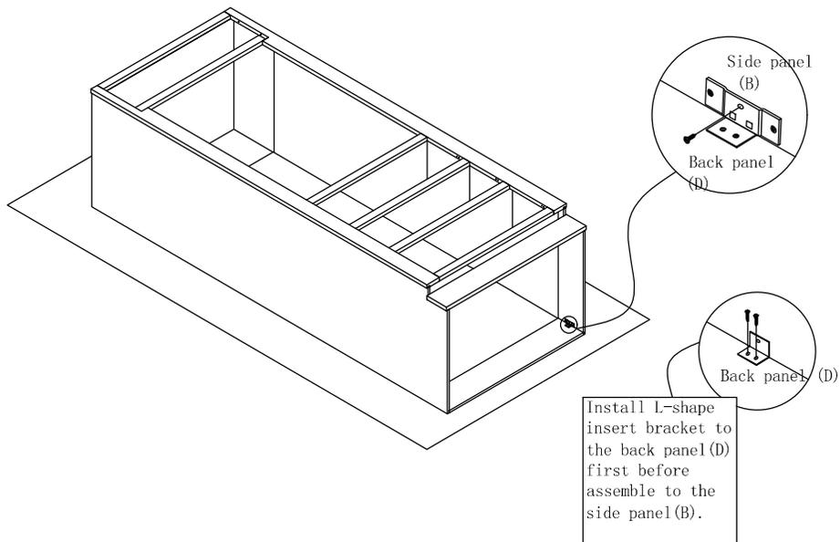
Step 8 : Install door panel (J) and corner block. screw the hing to the door and face frame, then install rainbow bracket to the side panel (B), front frame (A) and back panel (D) with the (4)  $\varnothing 3.5 \times 16 \text{mm}$  screw.
