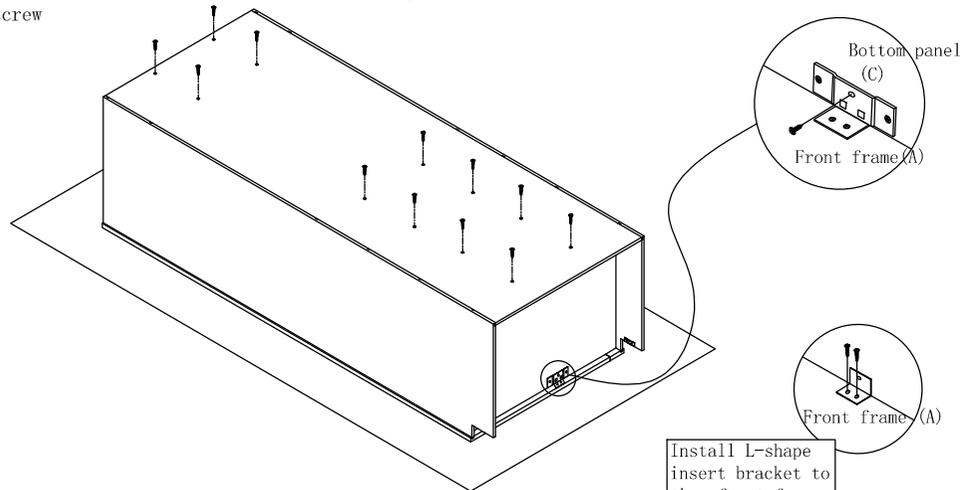
Install L-shape insert bracket to the front frame first before assemble to the bottom panel(C).
