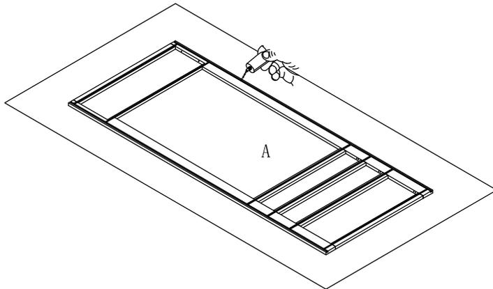
Step 2 : Install side panels. Insert side panel into groove of front frame (A) until side panel and front frame even.
