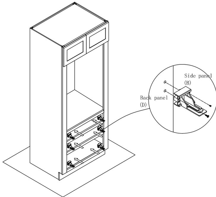
Step 10 : Insert drawer slide runner to the rear bracket and screw the drawer slide to guide hole of front frame and hole of drawer slide.
