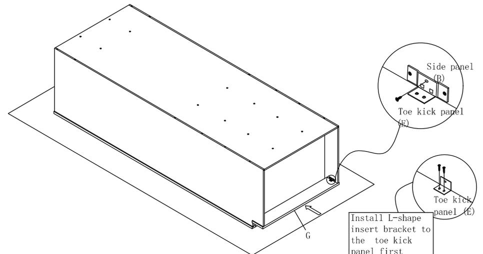
Install L-shape insert bracket to the toe kick panel first before assemble to the side panel(B).
