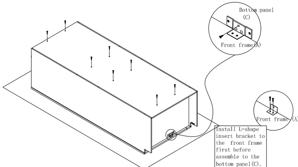
Step 6 : Install toe kick panel(G).Fit in the L-shape insert bracket from toe kick panel (G) into side panel (B) bracket and screw the bracket with (3)Ø3.5x14mm screw.
