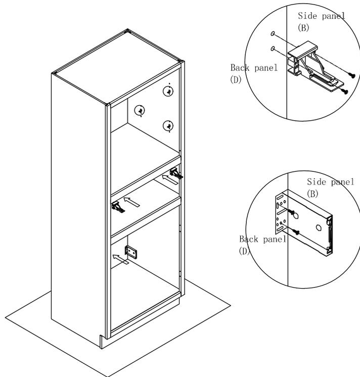
Step 10 : Install adjustable shelf(H) and drawer slide. Put the adjustable shelf on the shelf clips and Insert drawer slide runner to the rear slide bracket and screw the drawer slide to the guide hole of front frame (A) and hole for drawer slide, then screw the steel ball slide to the drawer side panel of drawer box.
