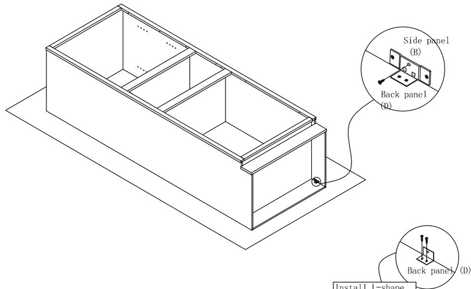
Install L-shape insert bracket to the back panel (D) first before assemble to the side panel (B).
