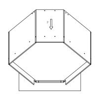
Step 6: Install assembly screws of back panel / side panels and connect panels.
