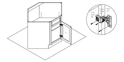
Step 12: Install overhead door hinge (7). Screw the overhead door hinge to the connection wood ( $\acute{6}$ ) and the drawer front ( $\acute{H}$ ), then install the overhead door hinge box to the drawer front
