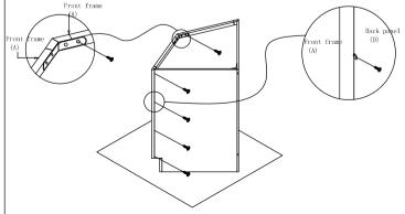
Step 6: Install toe kick panel. First connect two piece of toe kick with 135° bracket then assembly toe kick onto side panel (B) with (6) Ø4x25mm screw.
